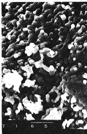
FIG. 2 Morphology of the Sample No 2 (Table I) after Reduction with Hydrogen Electron scanning microscope, magnification 10^4\times .
